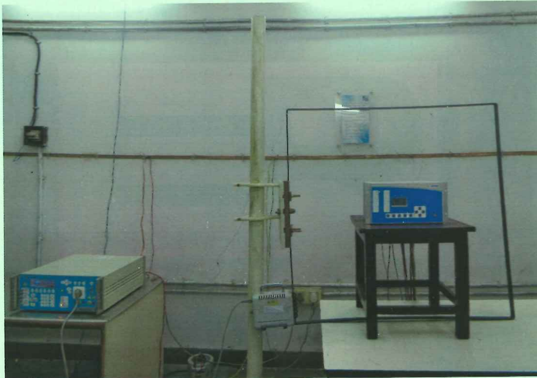
Test set up photograph for Power frequency magnetic field
